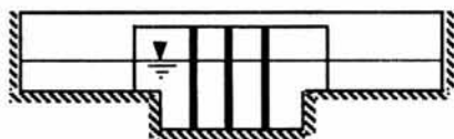
g) Single opening straight deck bridge model with piers (Bridge span width = 0.498m)
