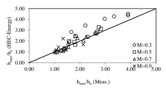
Fig. 3:Measured and Calculated (HEC-Energy) H<sub>max</sub>/H<sub>n</sub>values.
