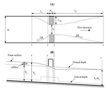
Fig. 1: Definition Sketch of Flow (A) Plan, (B) Profile Through A Bridge Waterway.
